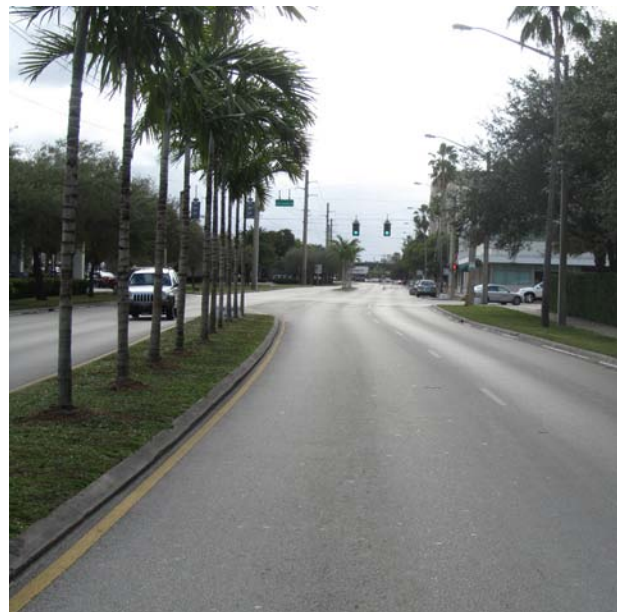
4. INCOMPLETE STREET Ponce de Leon is a great candidate for a complete streets makeover, with narrowed lanes, wide sidewalks, and a shade-tree lined median. The current palm trees are inappropriate as shade trees, while the sidewalks are non-existent on one side, and narrow on the other.
