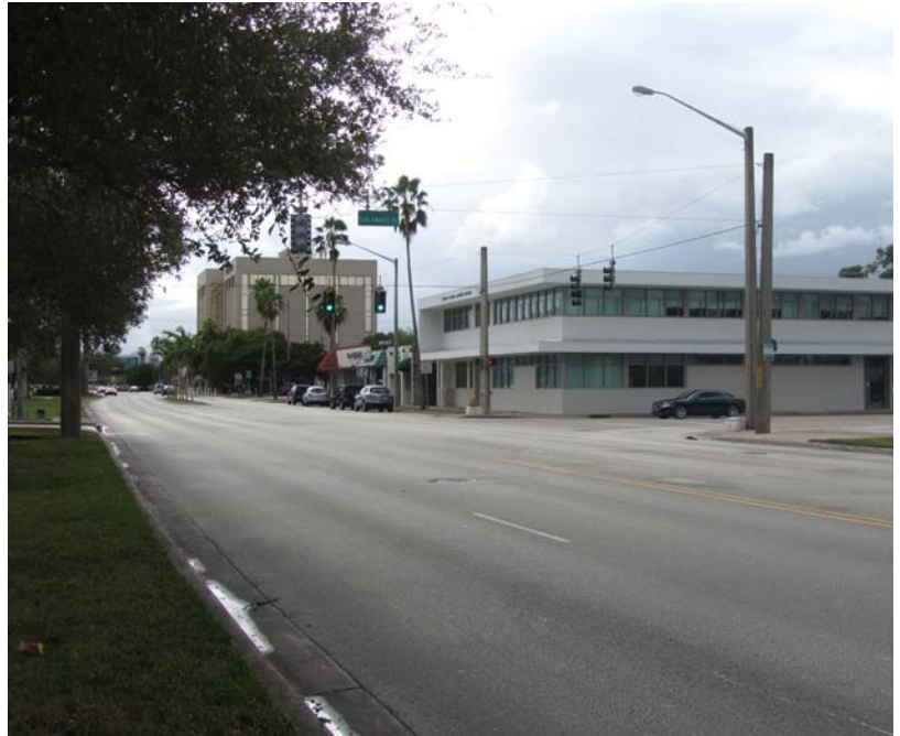
1. INTERSECTION This intersection has entirely too much pavement area to be a safe pedestrian crossing.
