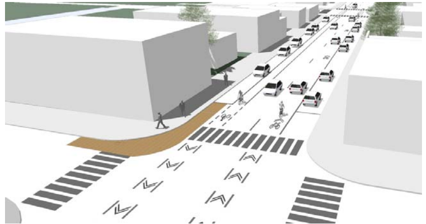
Peg-a-tracking should be used at intersections to continue the bike lane through the intersection
